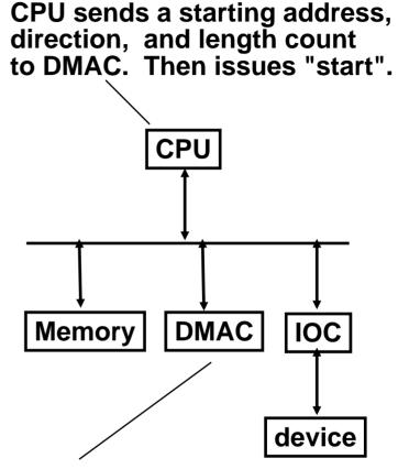
DMAC provides handshake signals for Peripheral Controller, and Memory Addresses and handshake signals for Memory.
