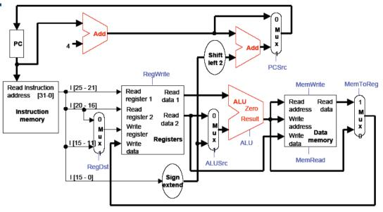
Remember we had to use a Harvard architecture with two memories to avoid requiring a memory that can handle two accesses in one cycle.
