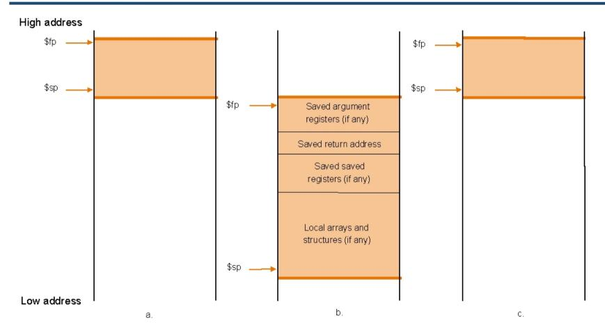
Stack pointer may change during the procedure, making procedure harder to understand Frame pointer offers a stable base register within a procedure for local memory references.
