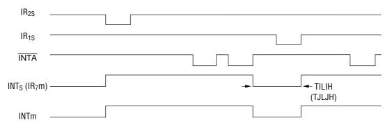
Fig. 3 Normal Operation Timing Chart
