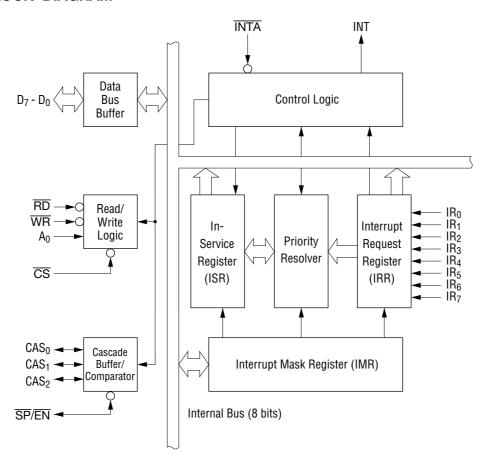
MSM82C59A-2 Internal Block Diagram
