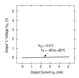
Note: The direction of flowing into the device is taken as positive for the output current.
