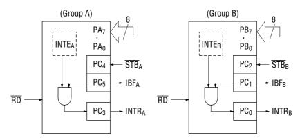
**Note:** Although belonging to group B, PC<sub>3</sub> operates as the control signal of group A functionally.
