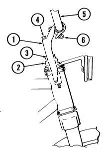
4. Tighten the stem bolt and the handlebar clamp:
