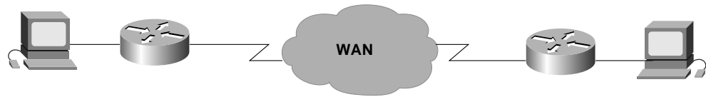
Figure 3-2 A Typical Point-to-Point Link Operates Through a WAN to a Remote Network
