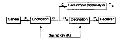
Figure 2.1: The information flow in a classical cryptographic system
