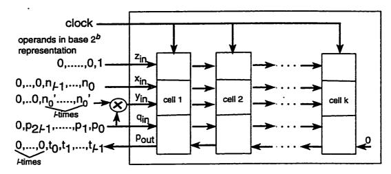
Figure 3.7: The systolic Montgomery reduction
