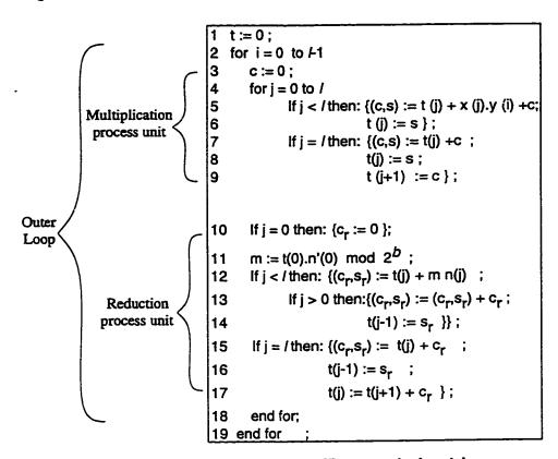
Figure 5.2: The reorganized MP merged algorithm
