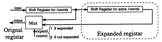
Figure 4.11: Expandable shift registers design
