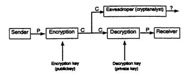
Figure 2.2: Public key cryptographic system (general concept)
