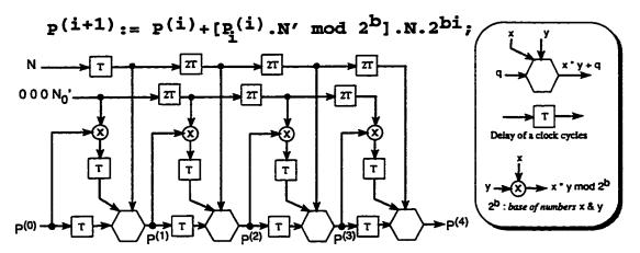
Figure 4.7: The signal flow graph MP implementation (parallel hardware)
