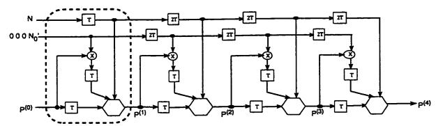
Figure 4.9: Projecting all parallel and systolic multipliers into one
