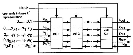
Figure 4.1: The word-serial multiplier (systolic array)
