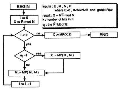
Figure 4.13: The Montgomery modular exponentiation algorithm
