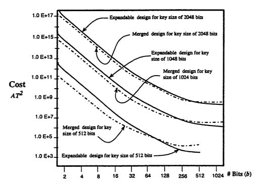
Figure 6.5: The expandable and merged designs costs for different key sizes
