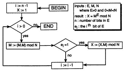
Figure 3.1: The repeated squaring algorithm
