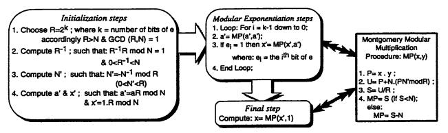
Figure 3.4: Montgomery's algorithm for modular exponentiation
