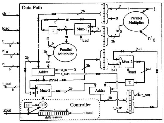
Figure 5.7: The reduction process implementation
