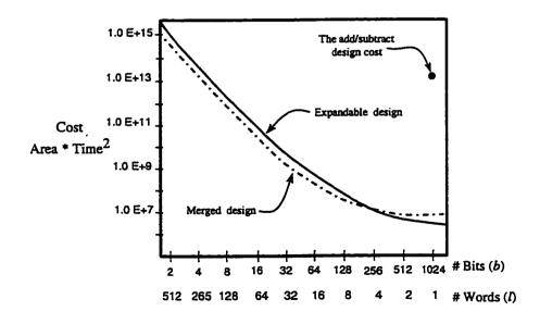
Figure 6.4: The Cost  $(Area * Time^2)$  analysis for key size of 1024-bits
