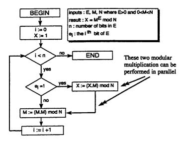
Figure 3.2: The improved repeated squaring algorithm
