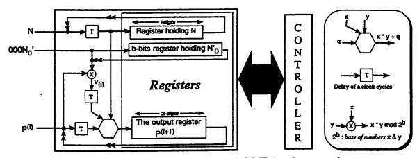
Figure 4.10: The expandable serial MP implementation
