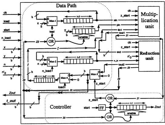
Figure 5.4: The merged MP multiplier implementation
