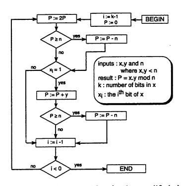
Figure 3.3: The multiplication with reduction modified algorithm
