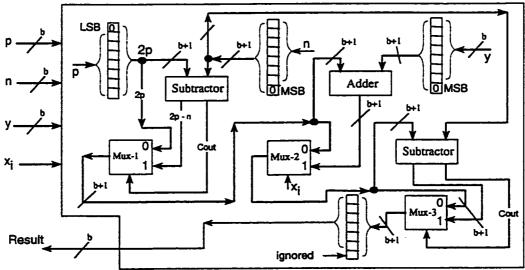
Figure 5.11: The modular add/subtract reduction implementation
