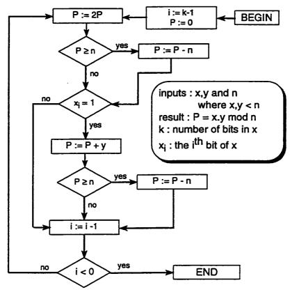
Figure 5.10: The add/subtract multiplication algorithm
