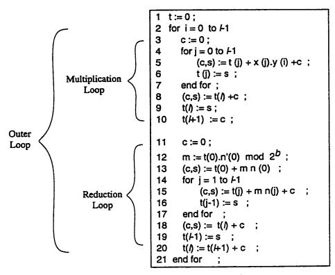
Figure 5.1: The MP merged algorithm
