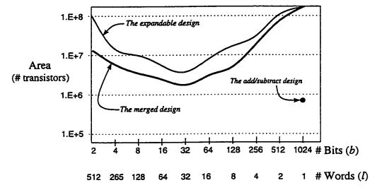
Figure 6.1: The area of the designs for key size of 1024-bits
