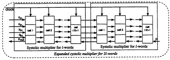
Figure 4.2: Expandability of the systolic multiplier
