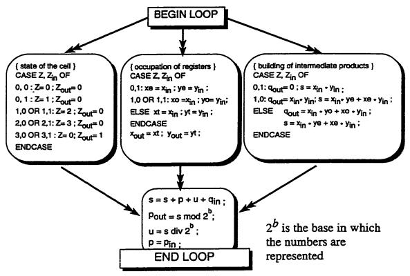
Figure 3.6: The algorithm for a cell behavior
