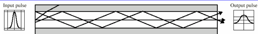
(a) Step-index multimode More than one path for signal – distortion Limits maximum data rate
