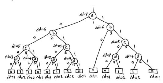
First, we set id(v) = 1 for all leaf vertices with value o and id(v) = 2 for leaf vertices with value l. We initialize ROBOD with two leaf vertices for o and l. Then, we process vertices at level 4, ire nodes with index = d.
