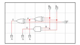
In order to construct a 4-bit CLA, four PFAs are needed to generate the signals that will be used in the functions below.
