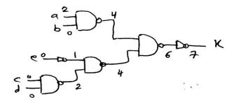
The maximum propagation delay in the optimized circuit is 7. The number of liderals in the original circuit is 11. The number of liderals in the optimized circuit is b. Thus, the area has also been reduced.
