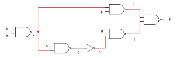
Assume that the delay of the inverter gate is 1 and that the delay of the 2-input NAND gate is 2. Also, assume that the input data-ready times are zero except for input *a*, which is equal to 2.
