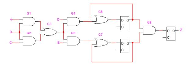
(i) Determine the critical path of this circuit and the maximum propagation delay.
