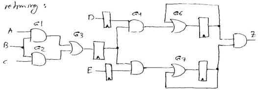
The maximum propagation delay in the resulting circuit is 4. The number of flip-flops has increased from 3 to 5.
