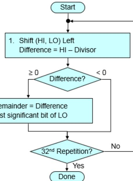
For our problem, the maximum value for the dividend is  $15*15=225$ . Thus, we will use an 8-bit divider where all the registers i.e., HI, LO, Divisor are 8-bits. The Quotient and Remainder will be taken from the least significant 4-bits of LO and HI registers, respectively. Note that it is possible to optimize the design by using only 5 bits for HI and Divisor and subtractor for our example.
