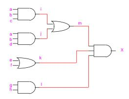
Assume that the delay of a gate is related to the number of its inputs i.e. the delay of a 2-input AND gate is 2. Also, assume that the input data-ready times are zero for all inputs.
