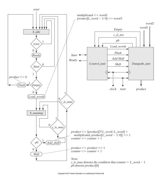
(i) Show the design of the data-path and control unit of the 4-bit sequential multiplier.
