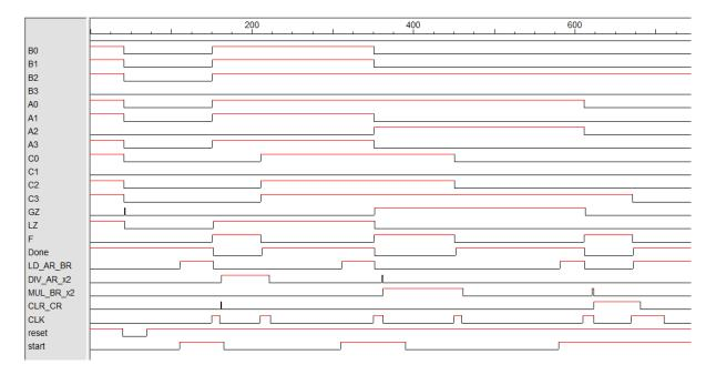
Simulation results above test the three cases and demonstrate correct operation of the circuit.
