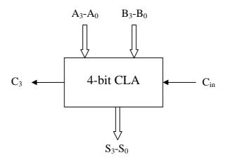
(i) Describe an Entity **CLA4** in VHDL for this 4-bit CLA using exactly the same port names shown above.
