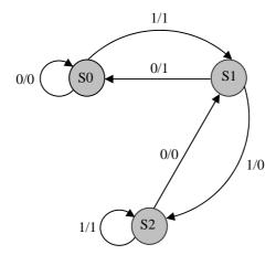
(ii) Model an Entity **Times3** and an Architecture **Behavior** for this circuit using a process. Assume that the circuit will have a synchronous reset and is rising-edge triggered.
