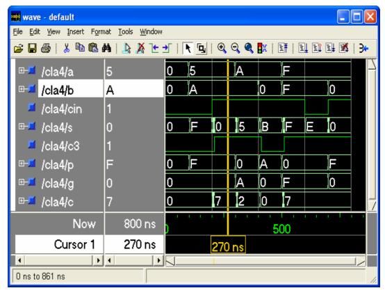
(iv) Model an 8-bit adder, **Adder8**, based on cascading two CLA4 components by connecting the carryout of the first component to the carry-in of the second component.
