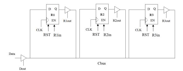
(i) Write a Verilog model **Datapath** to model the given datapath showing the inetrface signals assuming R1, R2, R3 as **output** signals, CLK, Reset, R1in, R2in, R3in, R1out, R2out, R3out, Dout and Data as **input** signals. Assume that RST is Asynchronous reset that resets the machine when set to 1. Use parametr n for determining the width of registers with a default value of 8.
