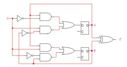
The machine is Moore machine as the output depends only on the current state and does not depend on the input. The next state and output equations are as follows:
