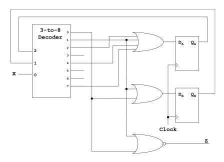
(i) Provide a state table for the given circuit showing the Present State, the input  $\mathbf{X}$ , the Next State, and the output  $\mathbf{Z}$ .
