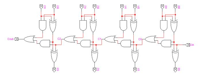
Determine and compute the **longest delay** in the **4-bit Ripple Carry Adder** (RCA).
