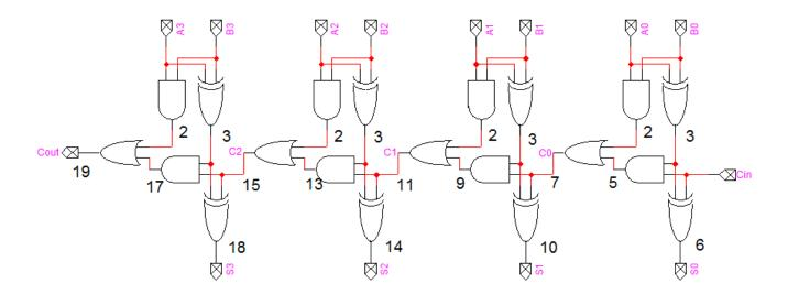
The longest delay is **19 ns** which is along the path from {A0 B0} across the propagate XOR gate until the Cout signal.
