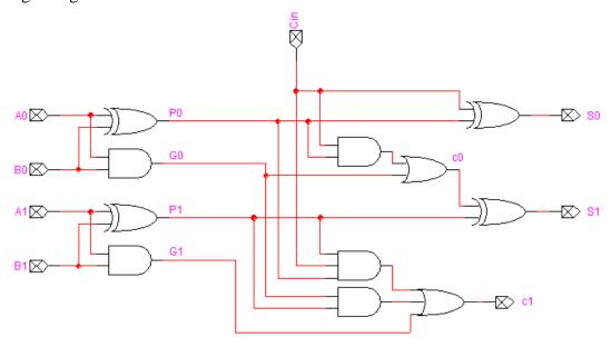
(c) (3 points) Using the delay assumptions given in the beginning of the question, determine and compute the <u>longest delay</u> in the 2-bit Carry Look-Ahead Adder (CLA).
