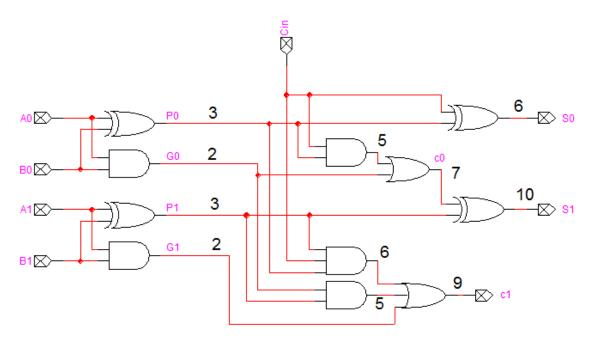
The longest delay is **10 ns** which is along the path from {A0 B0} across the propagate XOR gate until the S1 signal.
