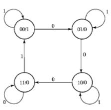
ii. Let the circuit be in state 00 with input X held permanently at 0. The circuit will end up being stuck at state 11. This state transition requires a minimum time duration of 1.5 ms.
