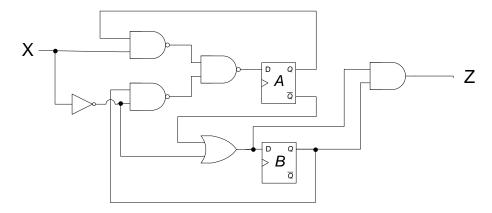
The circuit is Mealy since the output depends on both the current state and the input.
