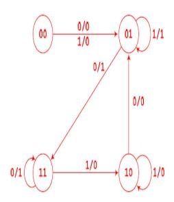
(ii) Complete the following waveform for the positive-edge triggered circuit that implements the state diagram provided below. Assume the circuit is initially at the state  $Q_1Q_0=00$ .
