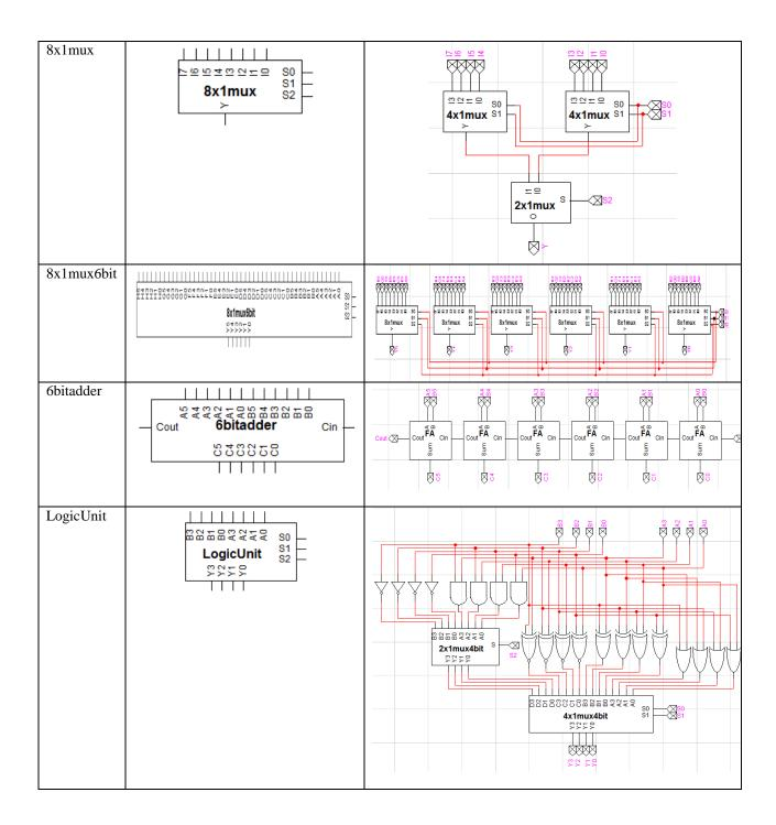
The whole ALU after integrating all the components and adding input and output is shown below:
