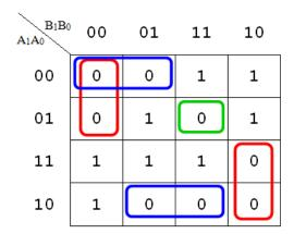
$$O_{1} = (A_{1} + A_{0} + B_{1})(A_{1} + B_{1} + B_{0})(\overline{A_{1}} + A_{0} + \overline{B_{0}})(\overline{A_{1}} + \overline{B_{1}} + B_{0})(A_{1} + \overline{A_{0}} + \overline{B_{1}} + \overline{B_{0}})$$
