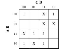
Q2. Implement the following circuit using only 2-input XOR gates with minimal number of gates:
