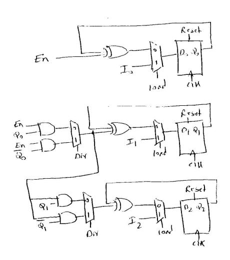
**Q.2.** Use the counter in  $(\mathbf{Q.1})$  to design a modular up/down counter that counts through the sequence  $\{0, 1, 2, 3, 4, 5\}$  up or down according to the signal Dir.
