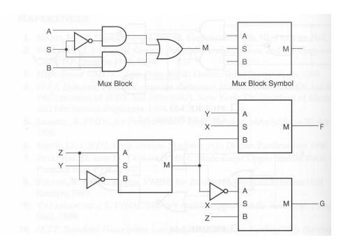
**Q.3.** Find the truth table for the outputs F and G of the hierarchical circuit shown below.
