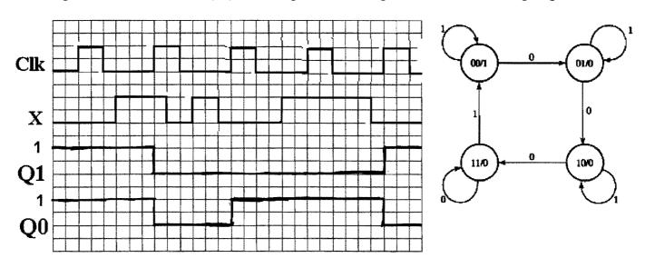
ii. Let the circuit be in state 00 with input X held permanently at 0. The circuit will end up being stuck at state 11. This state transition requires a minimum time duration of 1.5 ms.
