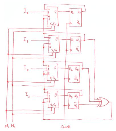
Note: It is possible to have any of the following connected to inputs 2 and 3 of the MUX that is connected to D<sub>3</sub>:
