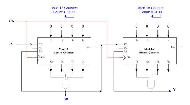
(II) Modify the counting system you designed in part (I) to make it self-resetting, i.e. whenever the system falls in any unused state, the count is automatically reset to zero. (3 Pts)
