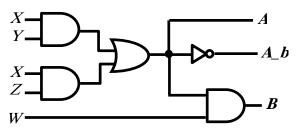
Assuming that all input/output ports have been declared properly; Write Verilog assign statement(s) to describe the circuit above (including worst case delays of the outputs). Outputs A\_b and B should be expressed as functions of the output A and other inputs.
