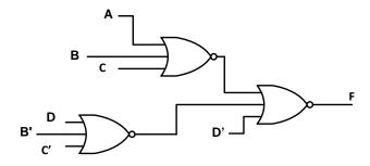
c. Assuming the availability of the true and complement of signals A, B, C, D and E, implement the shown circuit using minimum number of NAND gates only.
