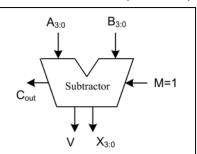
This **subtractor** can be used to compare both *unsigned* and *signed* 4-bit input numbers (**A** and **B**) by computing (**A-B**). It can be shown that the comparator output ( $A \ge B$ ) is given by:
