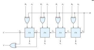
b. Given the FA circuit shown below, calculate the worst-case delay of this adder/subtractor circuit assuming gate delays as given in the table to the right.
