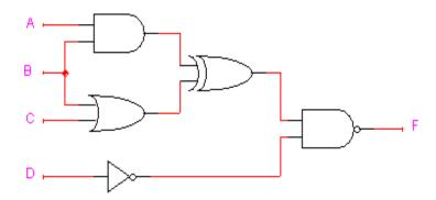
2. **(4 points)** <u>Using only NAND gates</u>, redraw the following circuit to show a multi-level **NAND** circuit. Only the **true** form of each input variable is available.
