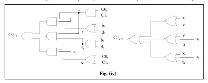
(I) Using the gate propagation delays of Table (i), what is the carry propagation delay *per single stage* for both of the output carries (C0 and C1)? (5 Points)
