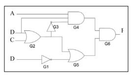
Critical Path Delay = G2+G5+G6=13 ns MAX Freq =  $1/(13x10^{-9}) = \approx 77MHz$
