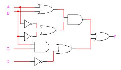
$$Y = (A + B)(\overline{A} + \overline{B}) + BC + \overline{D}$$
