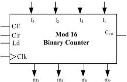
The counter should produce an output signal ( $C_{out}$ ) which equals 1 *only* during the last month of the year. (3 Points)
