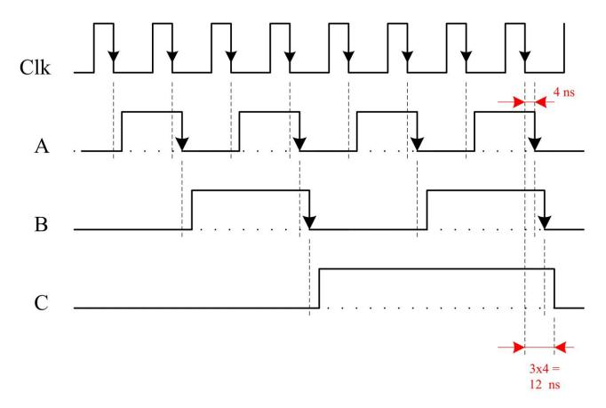
c. Assuming a negligible setup and hold times, an *inverter* delay of **1** ns and a delay from the *clock active edge till the new flip flop output* appearing of **4** ns, what is the <u>maximum clock frequency</u> at which the above circuit can operate? (**3 Points**)
