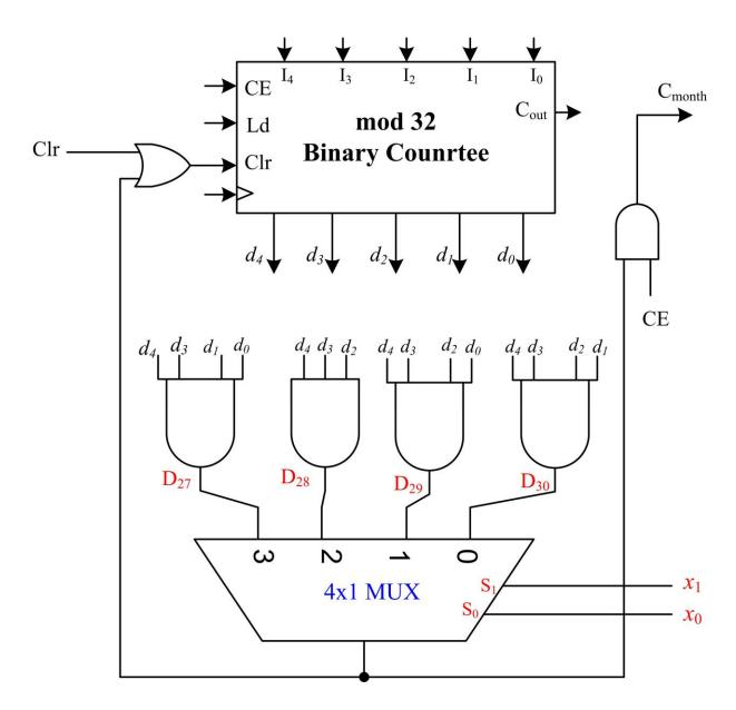
**c.** Given the output  $(m_3 m_2 m_1 m_0)$  of the *months* 'counter of part (a) and an input signal **L** that equals **1** only throughout leap years, derive the logic circuits which generate the signals  $x_I$  and  $x_0$  used by the *days* counter. (3 **Points**)
