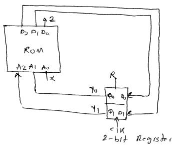
c. Starting at the initial state 00, what is the sequence of ROM location addresses that will be accessed when applying the input sequence X = 1100 where 1 is applied first. (2 points)
