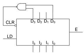
b. Add necessary gates to give the above decade counter cascading capability and then connect these decade counters together to build a three decimal digits counter to count from 000 to 999. (4 points)
