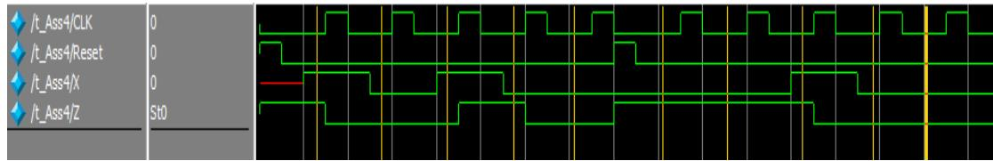
Looking at the waveform, one can see that the correct outputs are obtained for both applied input sequences as indicated by the shown cursors.
