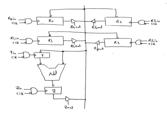
Note that the signals Rojont, Rlout, R2, out, and R3, out are derived from the signals Rsrc, out, Rdst, out and the conkent of IR. Similarly, Rdst, out and R0, in, R1, in, R2, in, and R3, in are the signals R0, in, R1, in, R2, in, and R3, in are derived from the signal Rdst, in and the content of IR.
