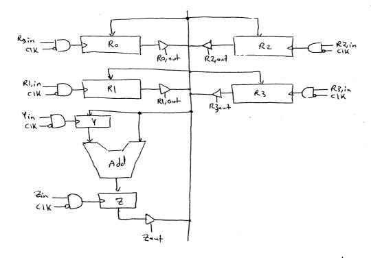
Note that the signals Roport, Rl, out, R2, out, and R3, out are derived from the signals Rsrc, out, Rdst, out and the content of IR. Similarly, the signals K0, in, R1, in, R2, in, and K3, in are derived from the signal Rdst, in and the content of IR.
