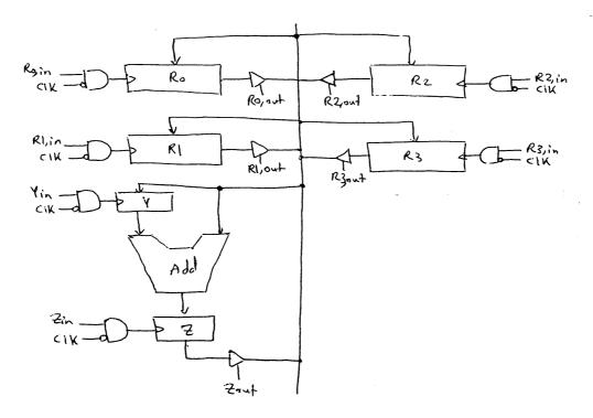
Note that the signals Roport, Rlout, R2, out, and R3, out are derived from the signals Rsrc, out, Rdst, out and the content of IR. Similarly, Rdst, out and the content of IR. Similarly, the signals 120, in, R1, in, R2, in, and R3, in are derived from the signal Rdst, in and the content of IR.
