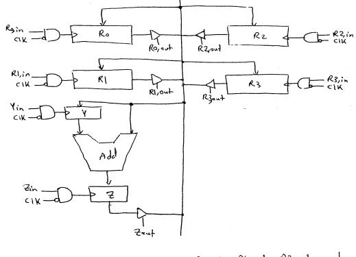
Note that the signals Ropout, Rhout, Report, and R3, out are derived from the signals Rsrc, out, Rdst, out and the content of IR. Similarly, the signals Ropin, Rhin, R2, in, and R3, in are derived from the signal Rdst, in and the content of IR.
