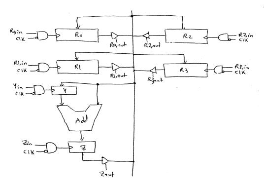
Note that the Signals Roport, Rl, out, R2, out, and R3, out are derived from the Signals Rsrc, out, Rdst, out and the conkent of IR. Similarly, Rdst, out and R0, in, R1, in, R2, in, and R3, in are the Signals R0, in, R1, in, R2, in, and R3, in are derived from the Signal Rdst, in and the content of IR.
