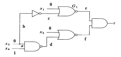
i. Using **Deductive fault simulation** technique, determine the set of faults detected by the test vector  $x_1x_2x_3x_4 = \{0001\}$ .
