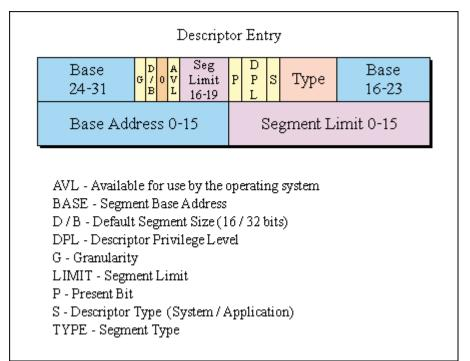
Figure 3 - Structure of a descriptor entry
