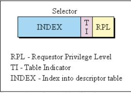
Figure 2 - Internal composition of a selector
