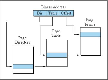
Figure 7 - Components of a linear address
