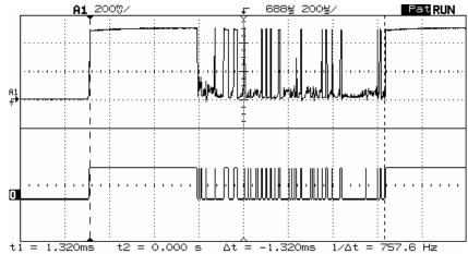
Switch Q – when released, it goes high for 480 µsec before generating 840 µsec of hash, a sure way to blow an interrupt system mad if poorly designed.
