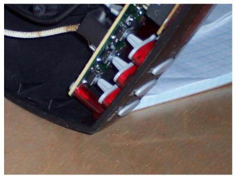
PCB switches in a cheap coffee maker.
