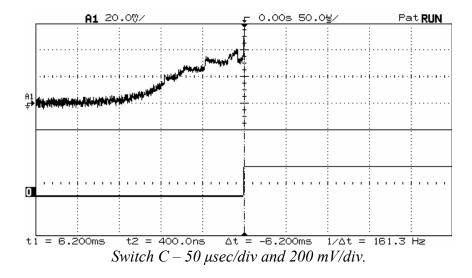
Another artifact of this wiping action was erratic analog signals treading in the dreaded no-man's land of TTL uncertainty (0.8 to 2.0 volts), causing the MSO to dither, tossing out ones or zeroes almost randomly, just as your microprocessor would if connected to the same switch.
