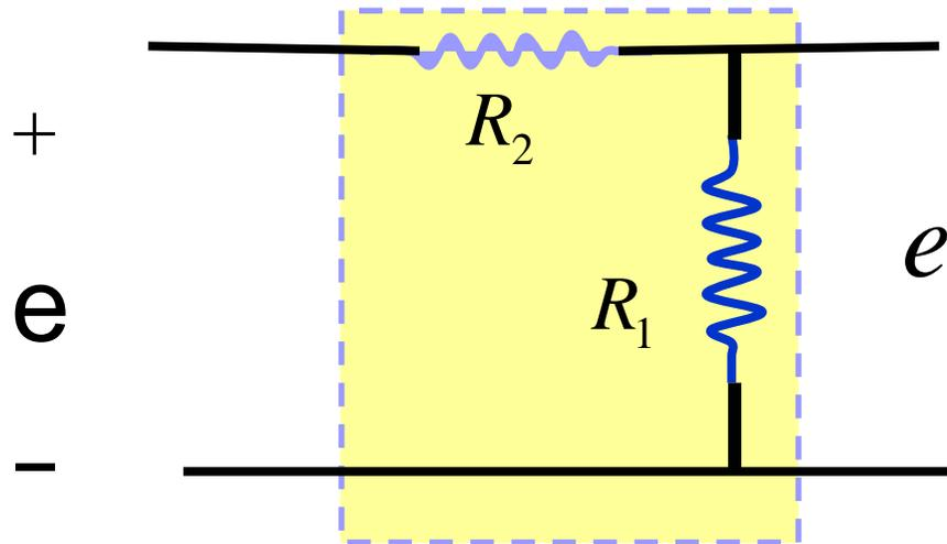
$$e_o = \frac{R_1}{R_1 + R_2} e,$$
