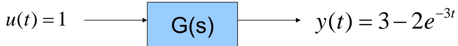
The **transfer function** can be obtained as the ratio of the Laplace transform of the output over the Laplace transform of the input
