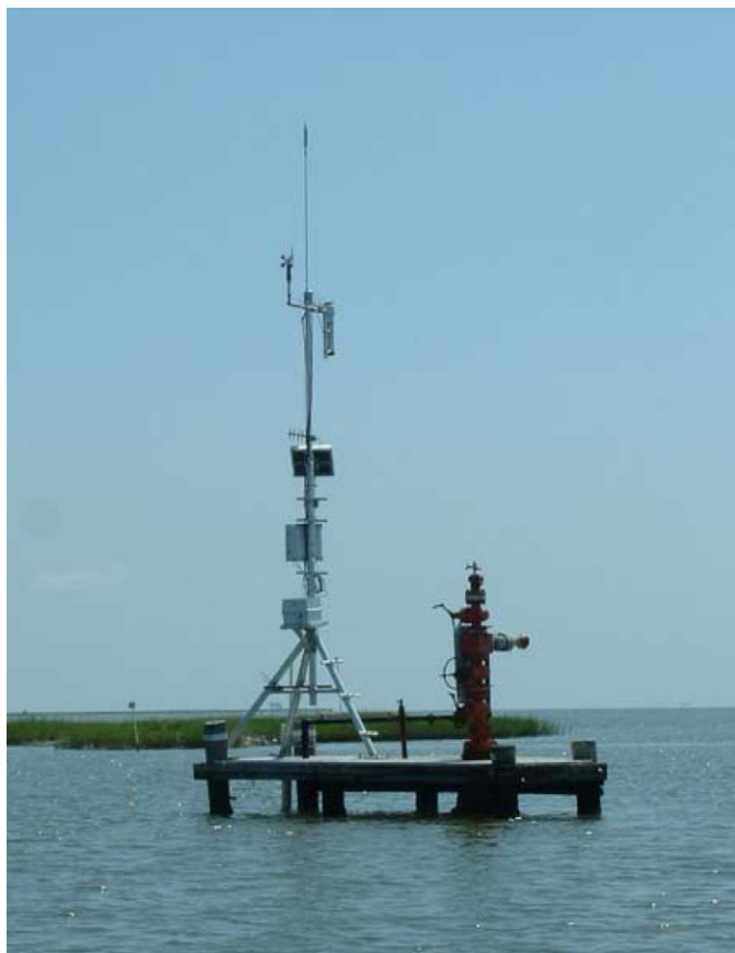
Fig. 9. Ocean observation system attached to an oil/gas structure. Source: LUMCON.
