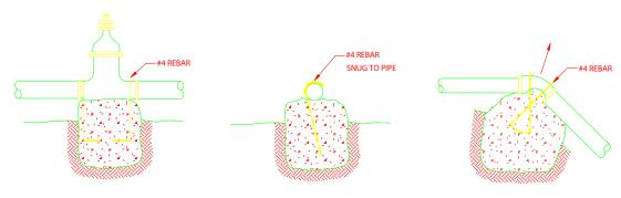
IF THRUSTS DUE TO HIGH PRESSURE ARE EXPECTED, ANCHOR VALVES AS ABOVE. AT VERTICAL BANDS ANCHOR TO RESIST OUTWARD THRUSTS.
