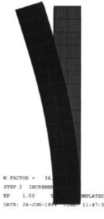
Figure 4: 3-dimensional contour model of the soil after a 10 kip force was applied to the pile. Note: the pile has been removed from this picture
