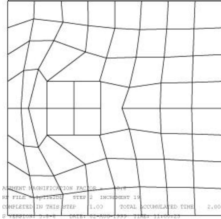
Figure 2: Two-dimensional model of 3 piles under lateral load with no gap created.
